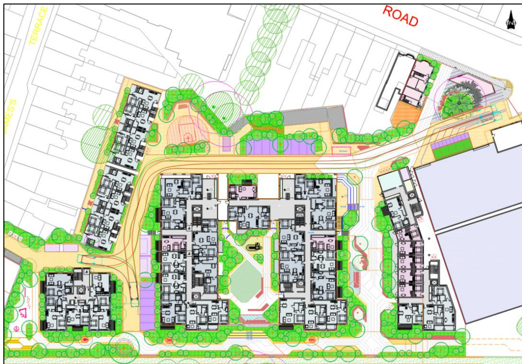
Figure 12: Auto Tracks of Refuse Vehicle Entering and Exiting
